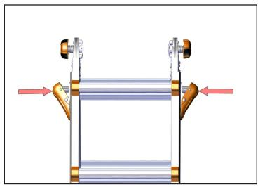
6. Re-engage Rock Lock tabs to lock the outer assembly to the inner assembly
